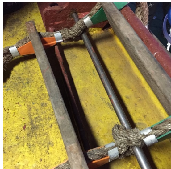
Fig 5: A steel bar used for securing the pilot ladder
