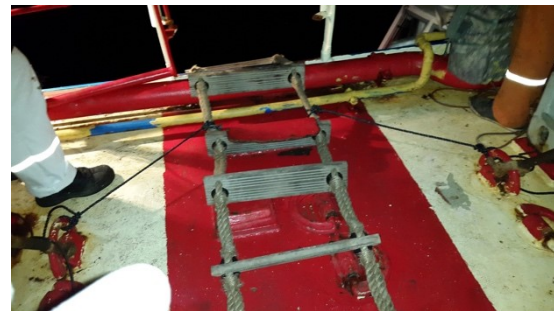
Fig 3: The shoestring method of securing
