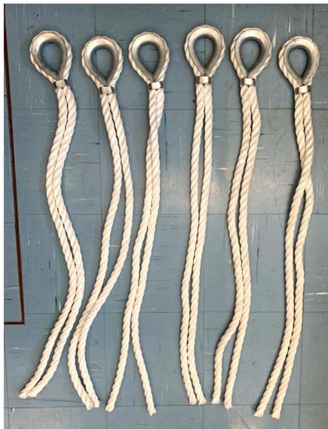
Figure 30: Examples of the polypropylene rope pairs provided for WP2 (manila pairs also provided).
