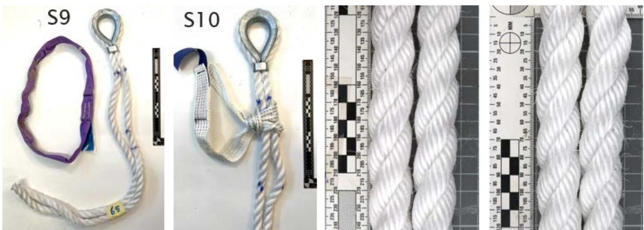
Figure 53: Scenarios 9 and 10 post-test (Left) and the examined worn section of the double rope (Right).
