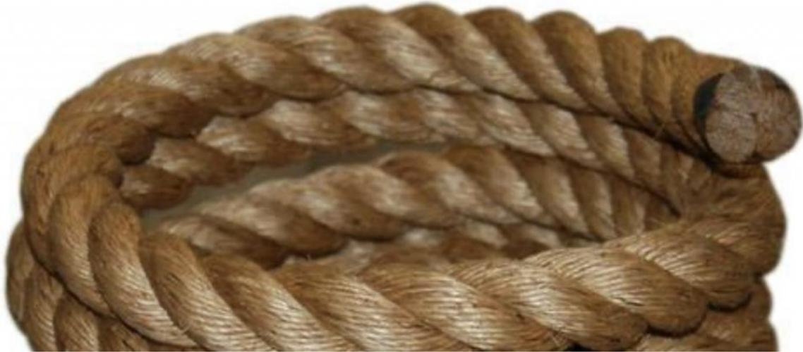
The ropes are the strongest part of the pilot ladder. Since the rope material is manilla rope, it is very vulnerable and sensitive to salt and water. Special care should therefore be taken when stowing the pilot ladder during the sea voyage.
