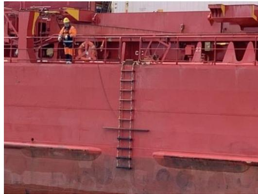
*Fendering is clear in way of the pilot ladder
