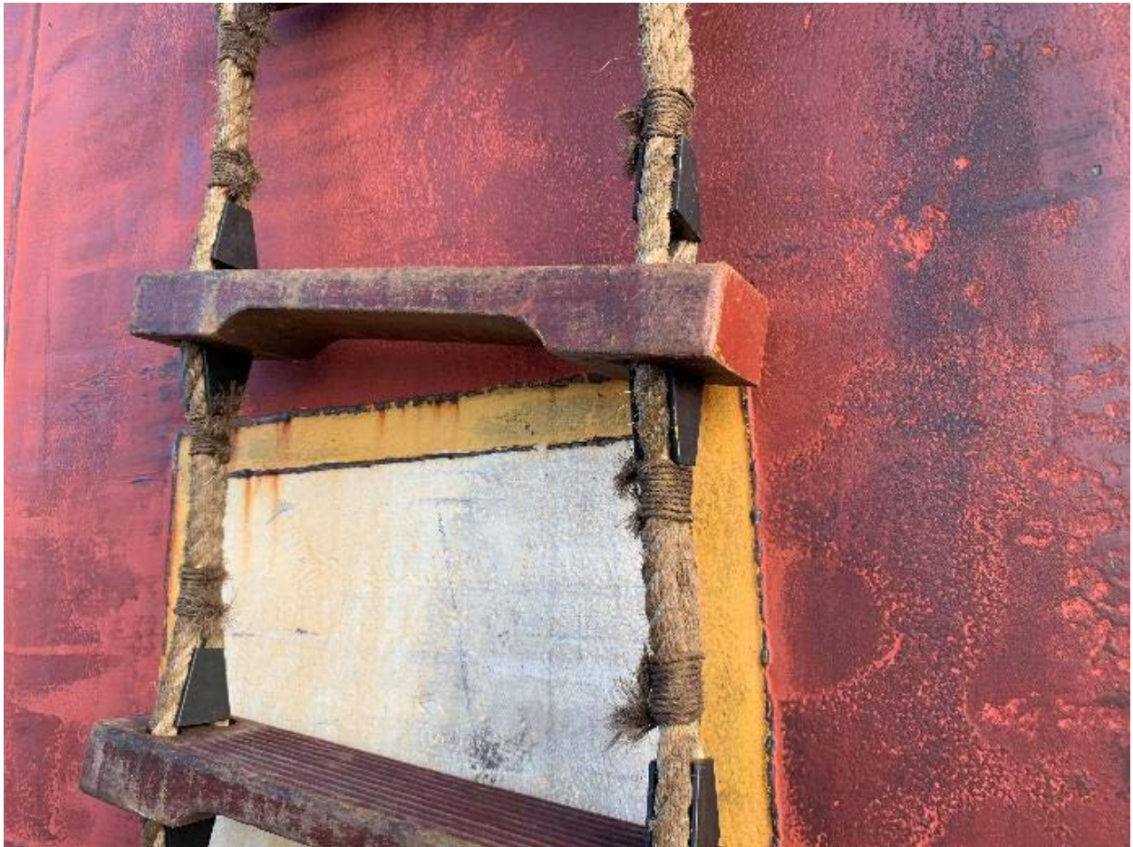
Loose steps due to worn out whippings.
