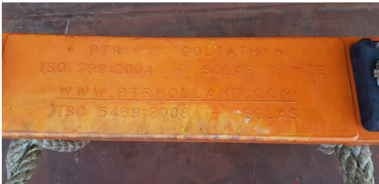
Marking under the step of the mentioned ladder
