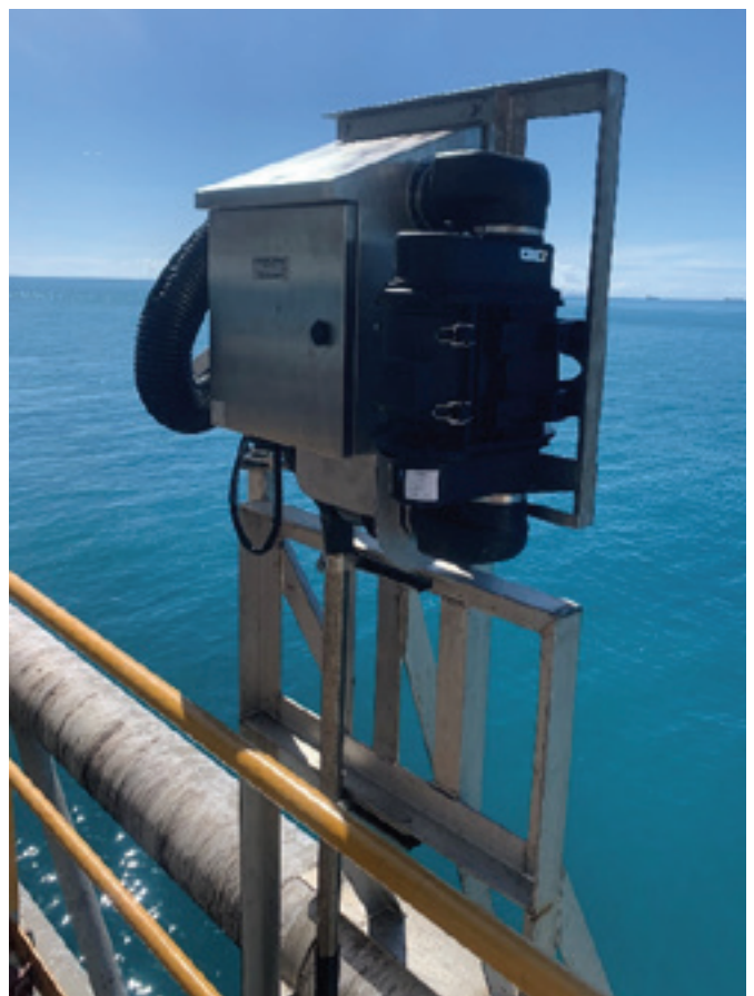
Figure 1. Docking Aid 3D sensor station permanently mounted on the wharf allowing the system to be always available without any manual setup required by pilots.
