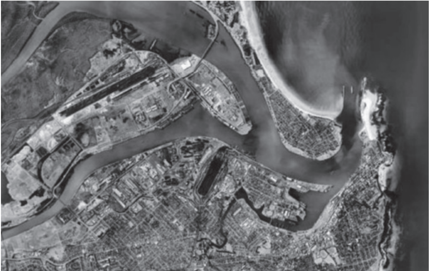
The port in 2002. Newcastle Port Corporation 2002 annual report. Note that the PWCS terminal has not been extended and NCIG does not exist. There is no Mayfield 4 and 7 berths and no passenger berth (channel berth).
