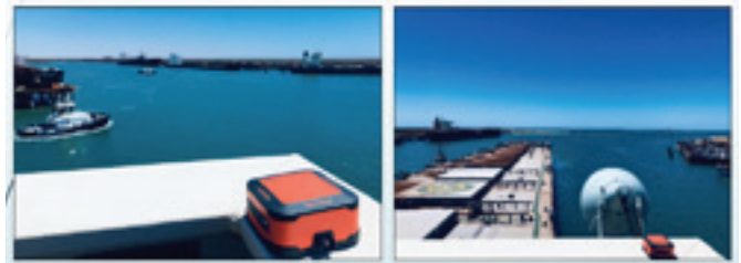
In Figure 5: convenient placement of port antenna and starboard antenna across the bridgewings on 55m separation baseline.
